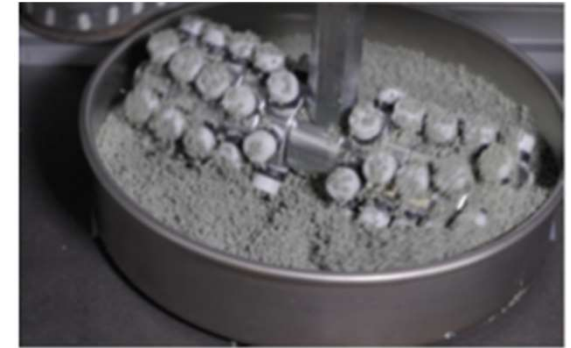
After 5 000 cycles On the left the reference sample and on the right the worn sample
