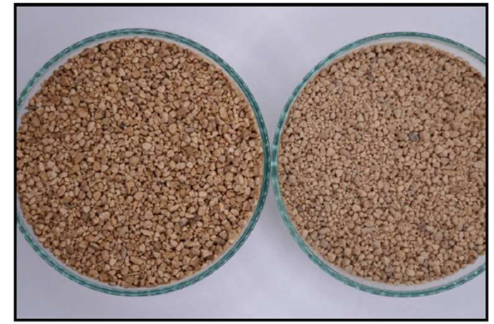
After 5 000 cycles On the left the reference sample and on the right the worn sample
